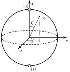
This is the famous **Bloch sphere**, which can be exploited to visualise single-qubit states and often helps to illustrate ideas about quantum computation and information, since it can be easily used to represent graphically the operations that can be performed on single qubits.
